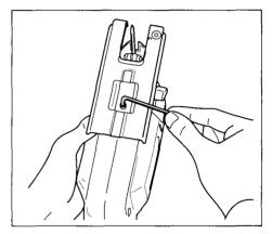
Loosen the bolt on the back of the base with the hex wrench and slide the base backwards. Tilt the base to the desired angle. The edge of the housing indicates the bevel angle.
